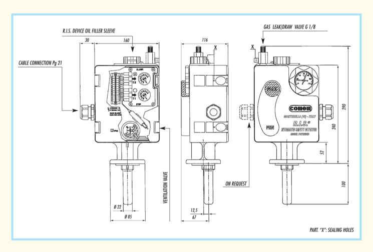
It is composed by a rugged plastic body, watertight and resistant to extreme climates, that houses a series of instruments and keeps under constant control the following operating conditions of the transformer:
